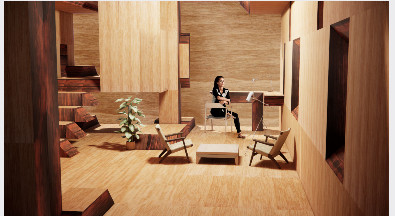
The interior can be left with the timber finish which provides a classy warm aesthetic. The exposed edges of the CLT are charred and treated with oil to seal it off. Similar treatment is provided for members on the exterior as well.
